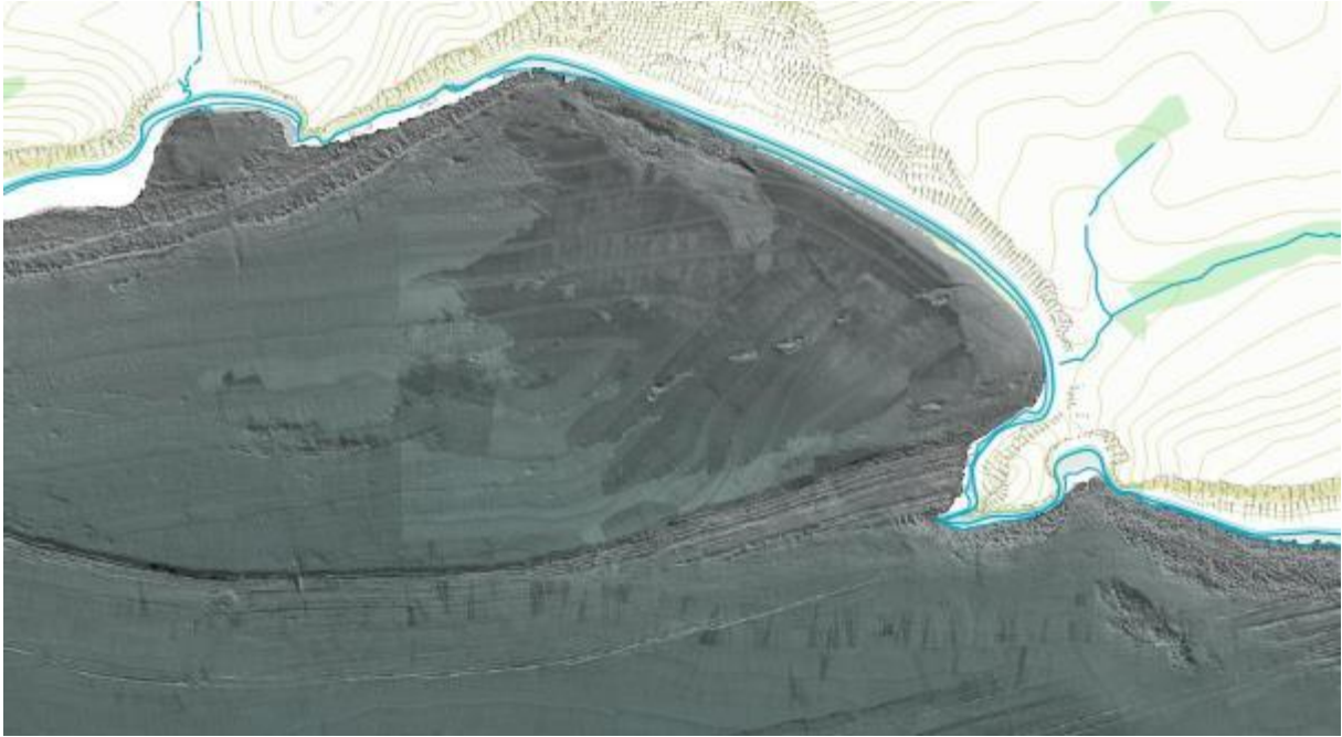
Figure 6: Bathymetry with multibeam backscatter overlaid. Contains Ordnance Survey data © Crown copyright and database right 2014. Contains MCA data ©Crown Copyright. Not to be used for navigation
