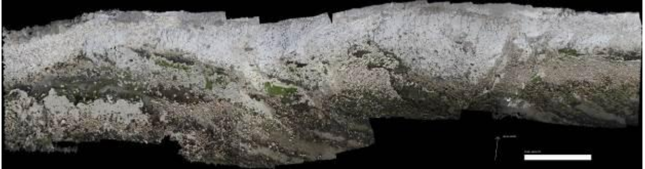
Figure 11 - 2mm resolution mosaic shot from a drone at 8m height. Covers 270m x 70m section of shore
