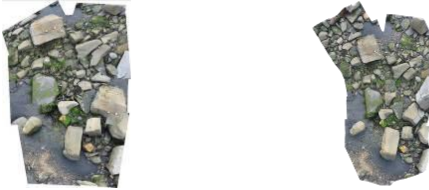
Figure 8 - Mosaic of 10 images of a rugged scene. The image on the left was created using Photoshop Merge, which is unable to cope with the parallax changes, the image on the right is orthorectified and was produced in PhotoScan
