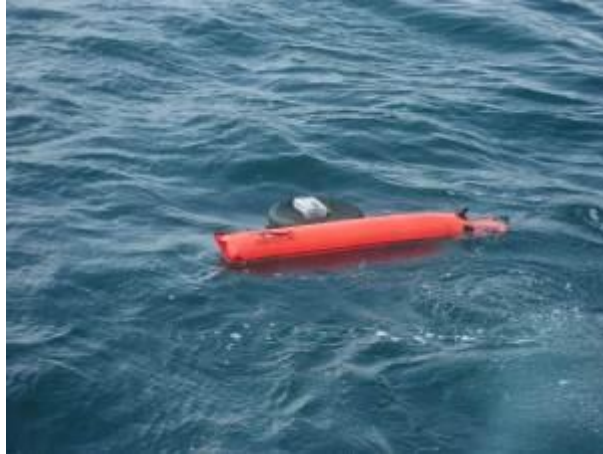
Figure 14 - Hand-held GPS unit in waterproof box fixed to inflated innertube and towed alongside SMB
